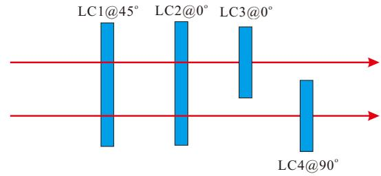
**Fig. 4. Realization of a single-photon operation on Alice's side.** The optical axes of the LCs are set at different angles, as shown in the figure. By applying different voltages, the LCs will introduce different phases between the fast axis and the slow axis.
