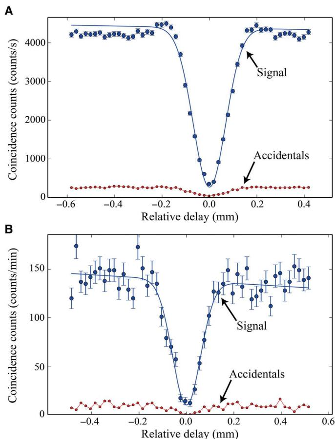
**Fig. 4. Measurements of indistinguishability.** (A) HOM interference of single photons using a commercially available fiber pigtailed 50:50 beamsplitter with a visibility of  $94.5 \pm 0.5\%$ . (B) HOM interference on the TBS with a visibility of  $93.1 \pm 2.8\%$ . The error bars shown are based on Poisson statistics.
