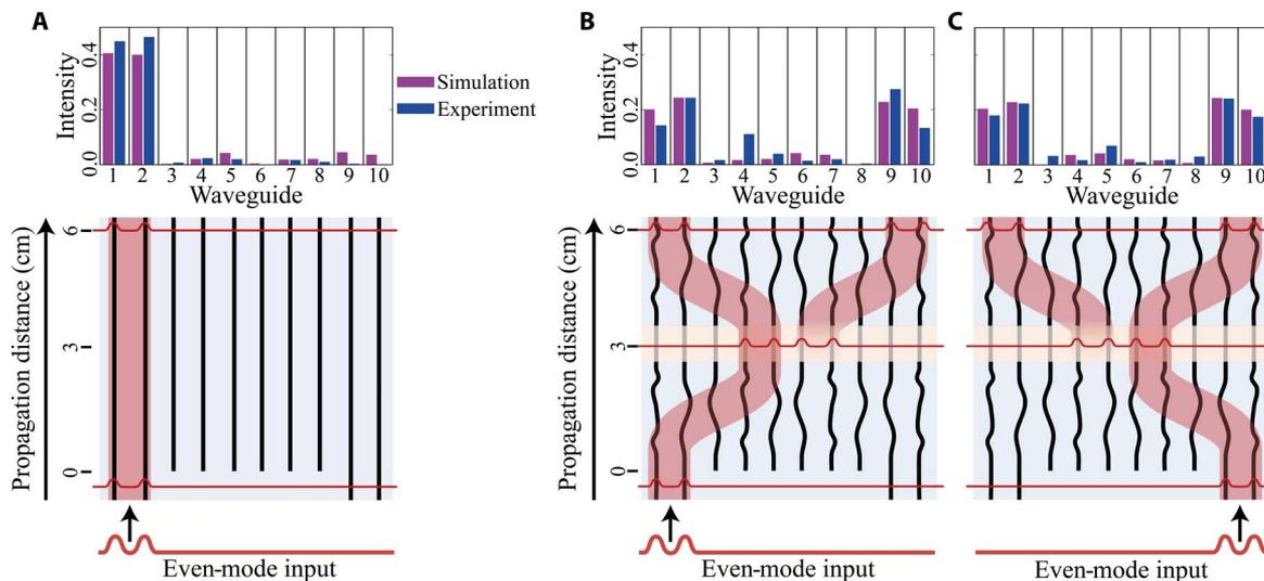
**Fig. 2. Characterization of the stationary boundary-state device and the TBS.** We characterized the output of the chip using laser light and a CCD camera. **(A)** The normalized output intensity distribution of the stationary boundary state. **(B and C)** The normalized output intensity distribution of the TBS with injection into the left and right inputs, respectively.
