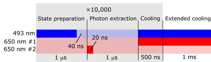
**Fig. 6. Experimental pulse sequence.** The experimental pulse sequence showing the timing of the laser beams used to state prepare, extract a single photon, and Doppler cool the ion. The parts of the sequence contained in the gray shading are repeated 10,000 times before an extended cooling cycle is performed.
