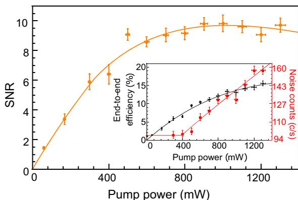
**Fig. 3. SNR measured after filtering of the frequency-converted ion signal.** The orange curve is the SNR given the measured conversion efficiencies and noise at each pump power. Inset: Measured conversion efficiency (black) and measured noise counts (red) on the APD as a function of pump power. The black curve is a theoretical fit to the efficiency data, and the red curve is an empirical fit to the noise.
