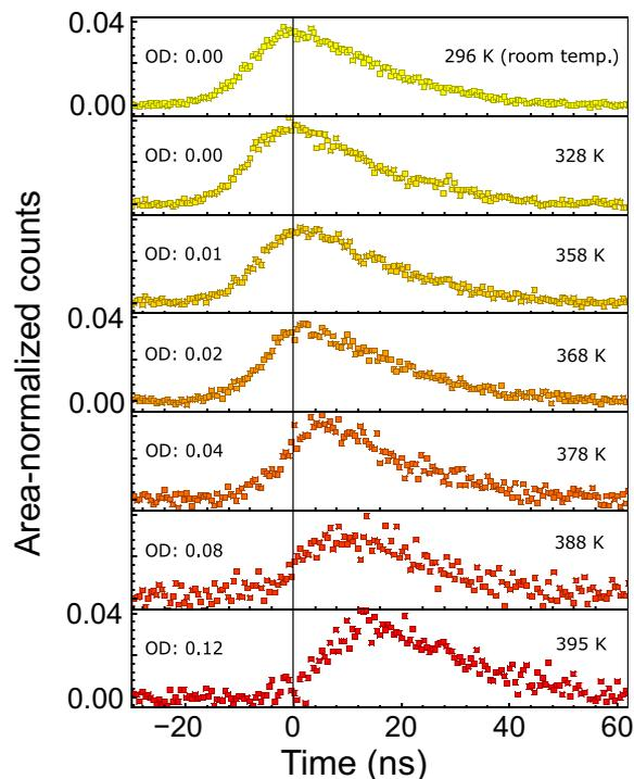
**Fig. 4. Area-normalized temporal photon shapes.** Area-normalized temporal shapes of frequency-converted photons that have passed through a warm  $^{87}\text{Rb}$  vapor cell. The  $^{87}\text{Rb}$  vapor cell temperature is set to the values indicated. The optical density (OD) of the warm vapor is stated for each temperature, at a frequency  $\omega_0$ , and using the same atomic density,  $N$ , used to fit the delay curve in Fig. 5.
