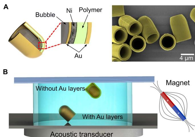
**Fig. 1. Schematic of the microswimmers and the acoustofluidic chamber.** (A) Schematic and false-colored scanning electron microscopy image of microswimmers (with Au layers). (B) Schematic of the acoustofluidic chamber. The microswimmers with and without the Au layer sink to the bottom or float to the top of the chamber, respectively.
