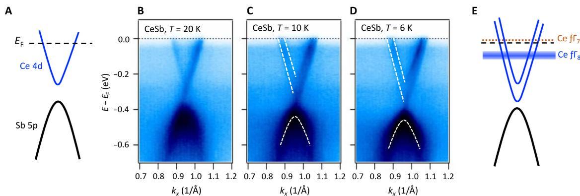
**Fig. 3. Observation of magnetic exchange splitting at X point.** Schematic of CeSb's band structure at X, (A) at  $T > T_N^0$  (E) at  $T < T_N^f$  (B to D) ARPES data taken at  $h\nu = 88$  eV near the X point for the selected temperatures (indicated at the top left). A clear signature of band splitting has been detected at  $T = 6$  K owing to Zeeman-like exchange splitting, which disappears above  $T_N^0$ .
