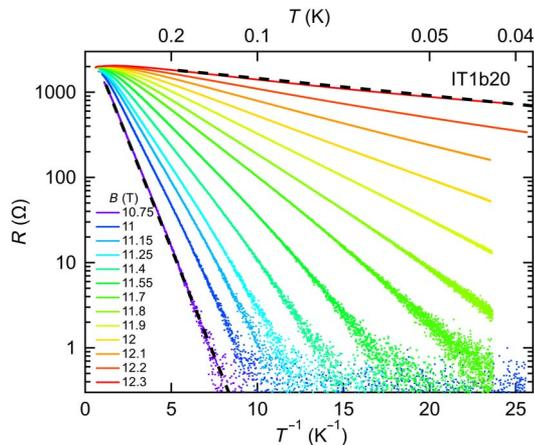
**Fig. 2. Fully recovered activated behavior.**  $R$  versus  $T^{-1}$  obtained from IT1b20, an a:InO film, measured with better filtration (see Materials and Methods for details) at different  $B$  values. Activated behavior (straight line in an Arrhenius plot) is apparent down to our noise floor or lowest measurement  $T$ 's (see, e.g., dashed black lines at  $B = 10.75$  and 12.3 T).
