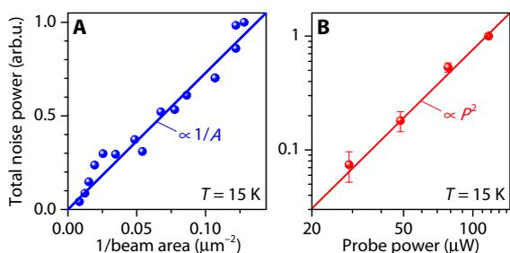
**Fig. 3. Dependence of the measured noise on probe parameters.** (A) The total (frequency-integrated) valley noise power scales as the inverse of the cross-sectional area  $A$  of the probe laser spot on the sample, as expected for optically detected noise measurements. (B) The total valley noise scales quadratically with the power  $P$  of the probe laser, again as expected for noise studies.
