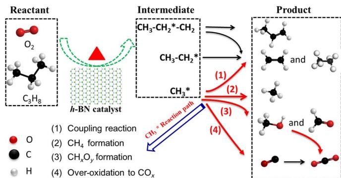
**Fig. 5.** The proposed reaction pathways of ODHP over the *h*-BN catalyst [using a structure model by Shi *et al.* (31) as an example].
