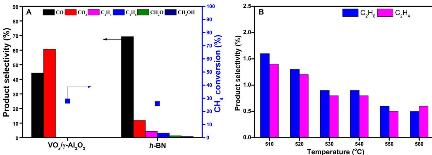
**Fig. 3. The product distribution of OCM and ODHP over the VO<sub>x</sub>/γ-Al<sub>2</sub>O<sub>3</sub> and h-BN catalysts. (A) Conversion and selectivity of OCM over the VO<sub>x</sub>/γ-Al<sub>2</sub>O<sub>3</sub> and h-BN catalysts. (B) Selectivity to C<sub>2</sub>-products (C<sub>2</sub>H<sub>4</sub> and C<sub>2</sub>H<sub>6</sub>) derived from the methyl coupling reaction in ODHP over the h-BN catalyst at different reaction temperatures.**
