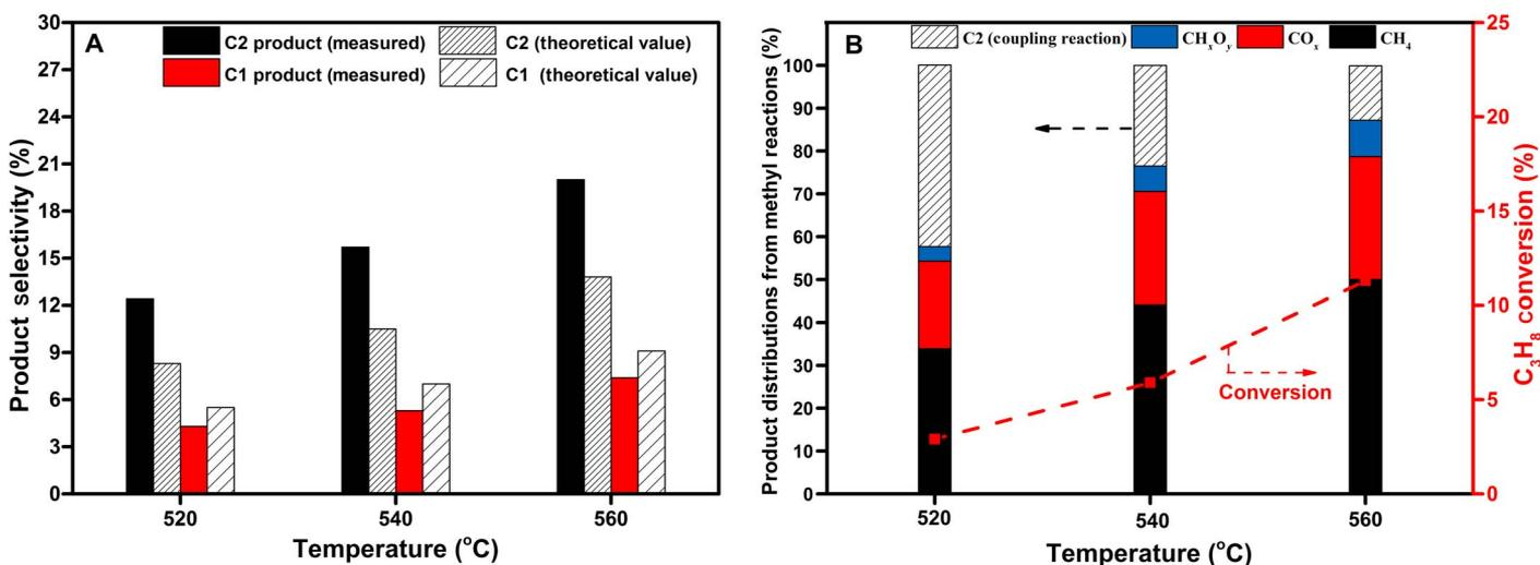
**Fig. 4.** The quantitative analysis of product from methyl reactions in ODHP over the *h*-BN catalyst. (A) Theoretical and measured selectivities of total C1- and C2-products. (B) Product distributions from methyl reactions in ODHP over the *h*-BN catalyst at different reaction temperatures.
