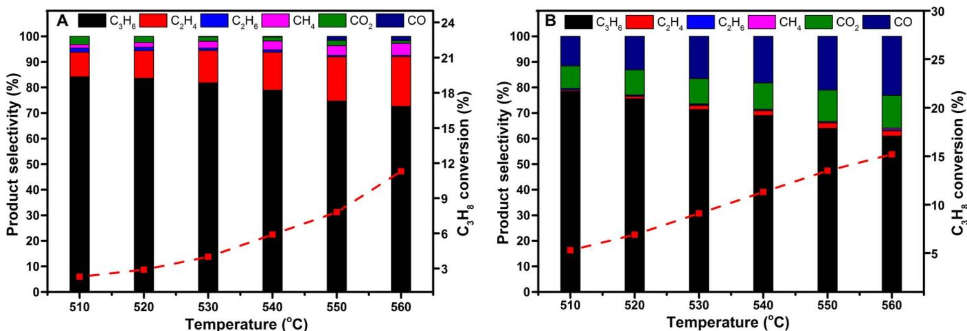
Fig. 1. The influence of reaction temperature on catalytic performance of ODHP. (A) *h*-BN catalyst; (B)  $\text{VO}_x/\gamma\text{-Al}_2\text{O}_3$  catalyst.
