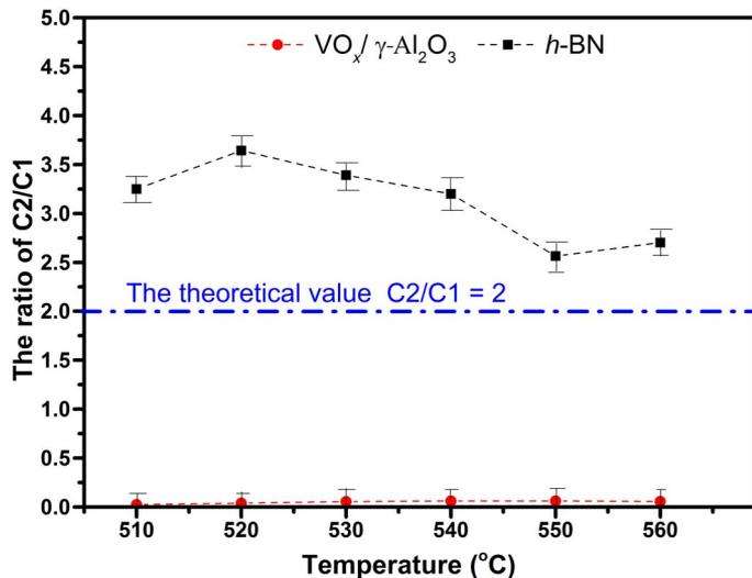
Fig. 2. Comparison of the C2/C1 ratio on the  $\text{VO}_x/\gamma\text{-Al}_2\text{O}_3$  and *h*-BN catalysts at different reaction temperatures.
