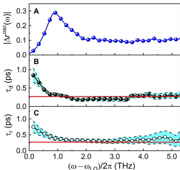
**Fig. 4. Coherent beat amplitude, dephasing, and reflectivity rise times.** (A) Amplitude of coherently oscillating component of the differential THz reflectivity. (B) The fitted dephasing time of the coherent oscillations and (C) the incoherent differential reflectivity rise time using the model discussed in the text. Shaded regions indicate 95% confidence regimes in the fitting. The red line in (B) and (C) marks one LO phonon period  $2\pi/\omega_{\text{LO}} = 270$  fs.
