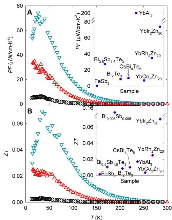
**Fig. 5. Temperature-dependent power factor and thermoelectric figure of merit of  $\text{YbTM}_2\text{Zn}_{20}$ .** Temperature-dependent (A)  $PF$  and (B)  $ZT$  of  $\text{YbCo}_2\text{Zn}_{20}$  (circle),  $\text{YbRh}_2\text{Zn}_{20}$  (up-triangle), and  $\text{YbIr}_2\text{Zn}_{20}$  (down-triangle). The insets in (A) and (B) are the  $PF$  and  $ZT$  values of several well-known thermoelectric materials at 35 K plotted together with parent compounds.
