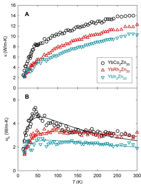
**Fig. 4. Temperature-dependent thermal conductivity of  $\text{YbTM}_2\text{Zn}_{20}$ .** Temperature-dependent thermal conductivity (A) and lattice thermal conductivity (B) for  $\text{YbCo}_2\text{Zn}_{20}$  (circle),  $\text{YbRh}_2\text{Zn}_{20}$  (up-triangle), and  $\text{YbIr}_2\text{Zn}_{20}$  (down-triangle). The solid lines are fits based on Eqs. 1 and 2 described in the text.
