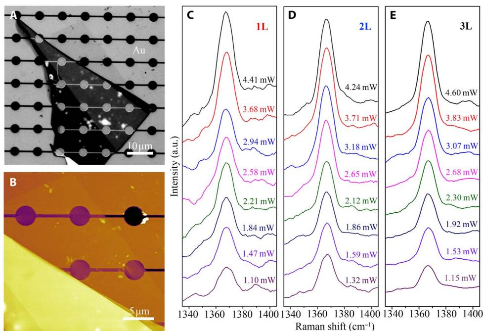
**Fig. 2. Laser power effect.** Optical (A) and AFM (B) images of a 1L BN on Au/Si. The Raman G bands of the suspended (C) 1L BN, (D) 2L BN, and (E) 3L BN under different laser power. a.u., arbitrary units.
