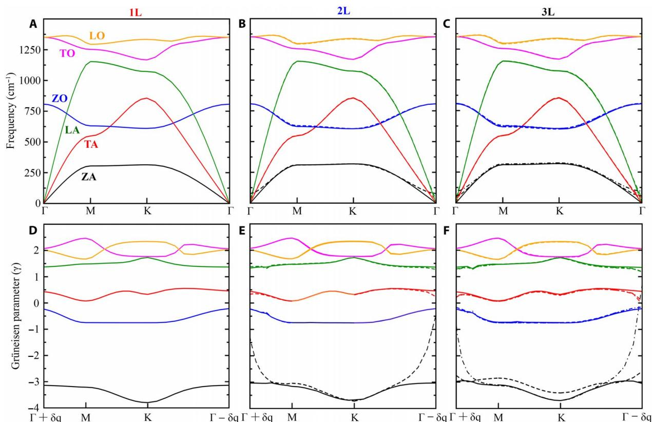
**Fig. 5. Phonon dispersion and Grüneisen parameters.** (A to C) Phonon dispersion and (D to F) Grüneisen parameters of 1-3L BN calculated by DFT. The phonon branches are labeled for 1L BN. Dashed curves represent additional phonon branches and corresponding Grüneisen parameters due to additional BN layers.
