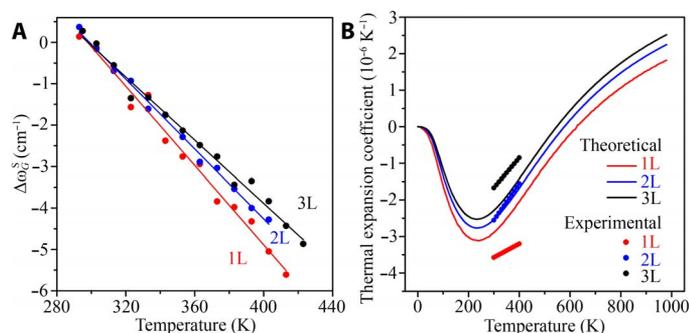
**Fig. 6. TECs of 1-3L BN.** (A) The G band frequency shifts as a function of temperature and the corresponding fittings of 1-3L BN bound to SiO<sub>2</sub>/Si using TECs as fitting parameters. (B) Experimental (dots) and theoretical (lines) curves of the TECs of the 1-3L BN.
