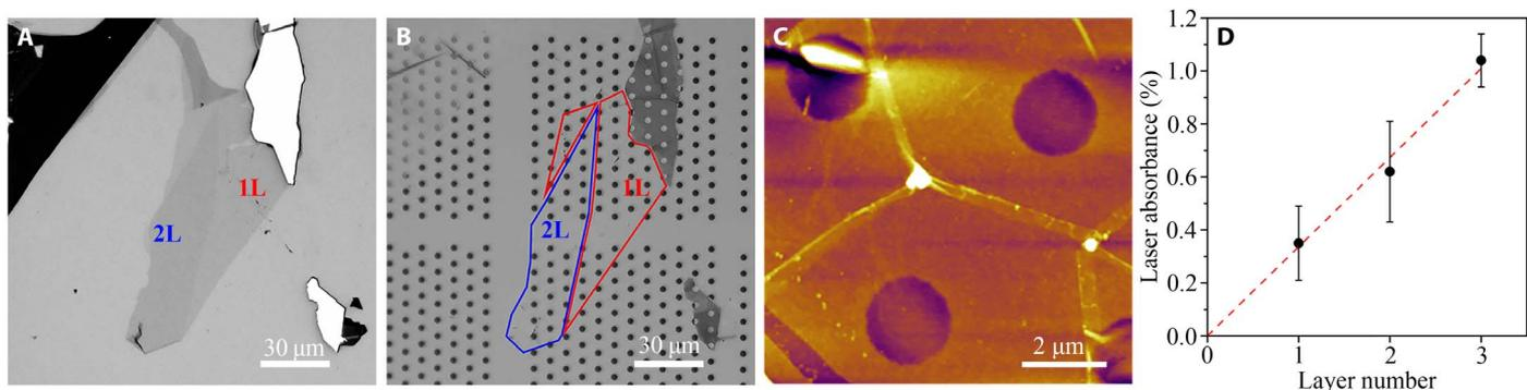
**Fig. 3. Light absorbance of atomically thin BN.** Optical images of a 1-2L BN as exfoliated on SiO<sub>2</sub>/Si (A) and transferred onto a Si<sub>3</sub>N<sub>4</sub> TEM grid (B). (C) AFM image of the BN suspended over the TEM grid. (D) Laser absorbance of 1-3L BN and the corresponding linear fitting.
