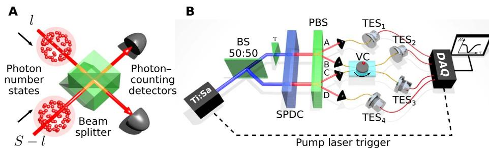
**Fig. 1. Photonic implementation of a fractional QKT.** (A) HOM interference of photon number states on a variable BS, followed by two photon-counting detectors, (B) Setup: Ti:Sa, titanium-sapphire laser pump (blue); BS, 50:50 BS;  $\tau$ , optical phase delay; SPDC, periodically poled potassium titanyl phosphate nonlinear spontaneous parametric down-conversion waveguide chip that produces photon number-correlated states (red); VC, variable coupler; DAQ, data acquisition unit.
