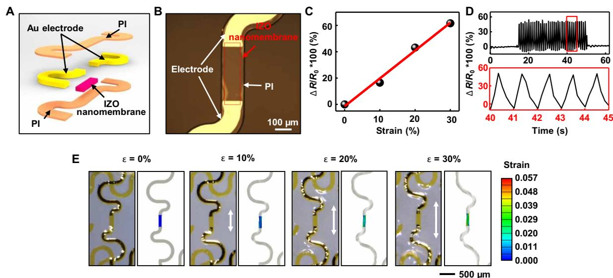
**Fig. 4. Characteristics of strain sensor.** (A) Schematic exploded view of the IZO strain sensor. (B) Optical microscopic image of the strain sensor. (C) Calibration curve of the strain sensor. (D) Relative resistance change of the strain sensor under cyclic stretching and relaxing. (E) Sequential images of the strain sensor under strain and corresponding FEA results of IZO.
