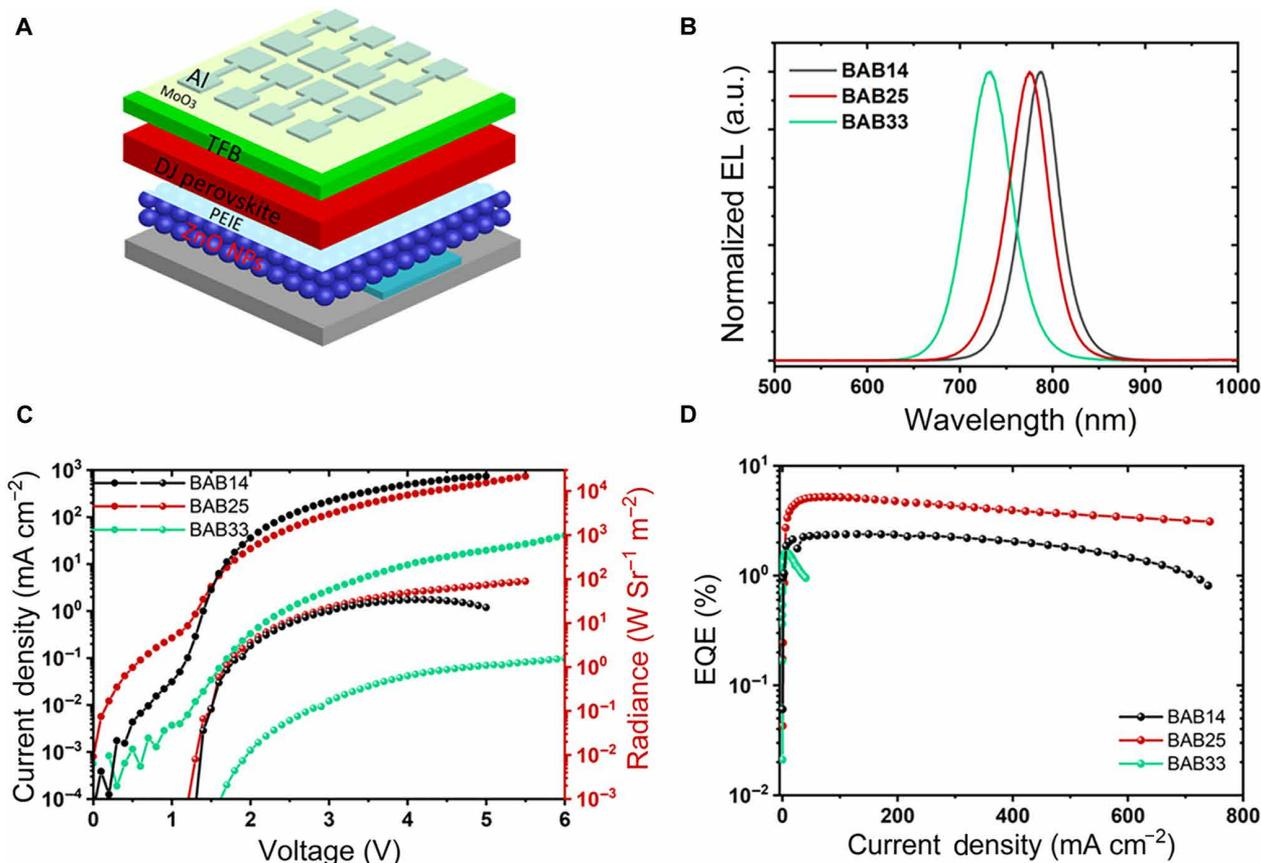
**Fig. 5. Characteristics of DJ structure perovskite LEDs.** (A) Device structure. (B) Normalized electroluminescence spectra of hybrid DJ structure perovskite LEDs with varied ligand additive. (C) Current density–voltage–radiance curves and (D) EQE curve of hybrid DJ structure perovskite LEDs.
