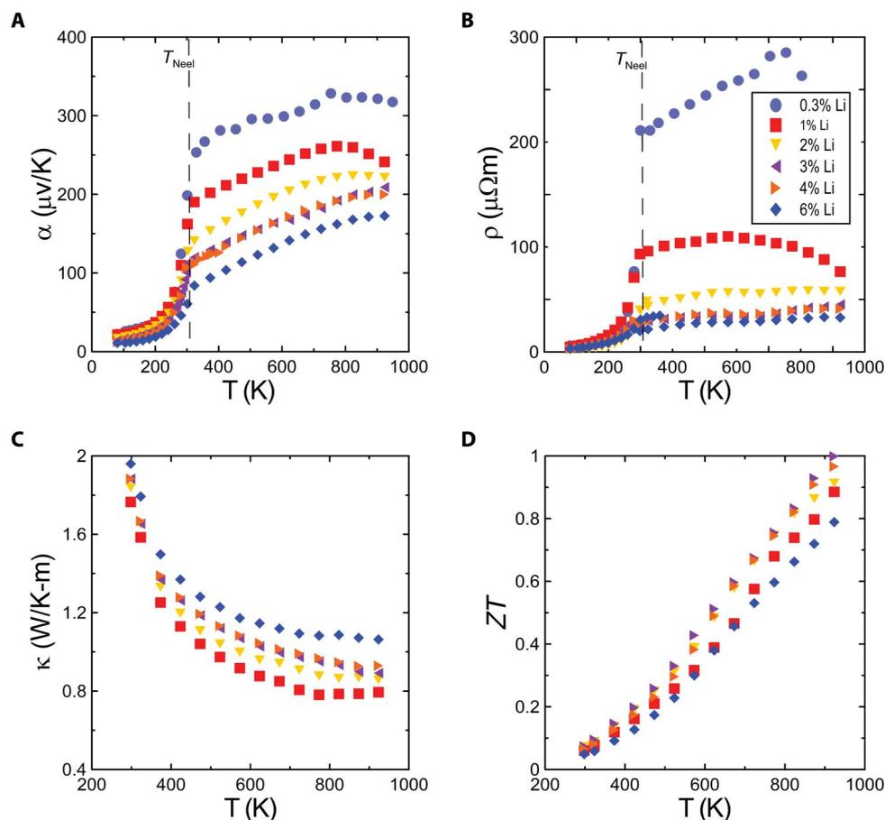
**Fig. 1. Transport properties of Li-doped MnTe.** (A) Thermopower, (B) resistivity, (C) thermal conductivity, and (D) thermoelectric figure of merit  $ZT$ . The Li concentrations for all frames are shown in the inset of frame (B).
