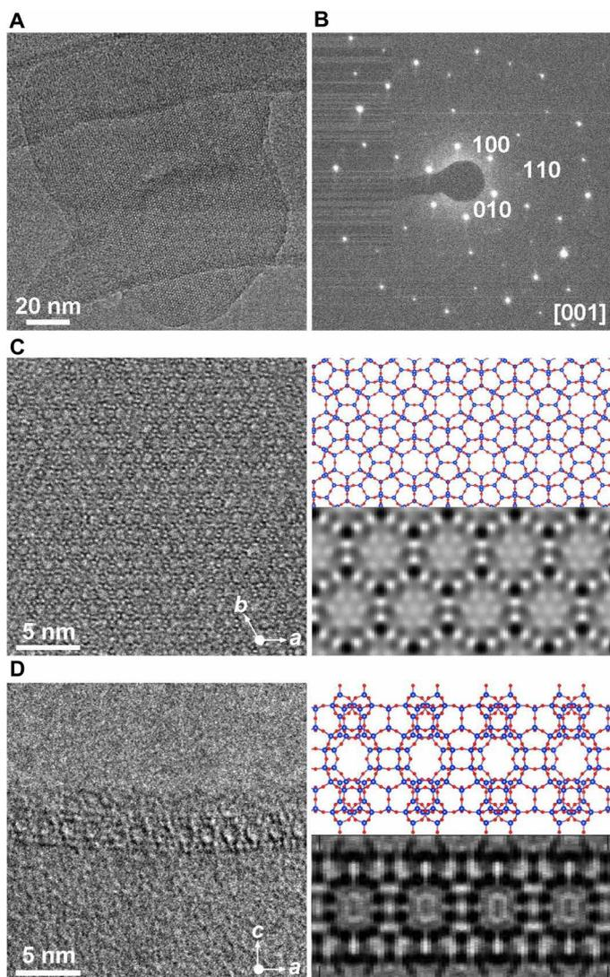
**Fig. 3. Crystalline structure of MCM-56 monolayers separated from the colloidal suspensions.** (A and B) TEM image and SAED pattern along the *c*-axis, showing the whole nanosheet to be a single crystal. (C and D) HRTEM images, atomic models, and simulated TEM images of in-plane (C) and edge-view (D) structures.
