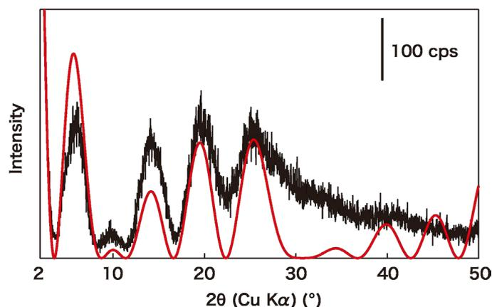
**Fig. 1. In situ XRD of concentrated layers in water (black line) and the square of structure factor  $F$  (red line) calculated based on the MWW structure.** The observed deviation between the calculated and experimental intensities at higher  $2\theta$  angles is due to amorphous halo from water because the glue-like sample recovered via centrifugation contains large amount of the solvent. Damping the wavy profile at a higher angular range may be involved by some structural disorder.
