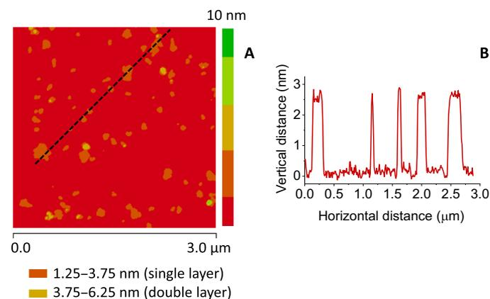
**Fig. 2. AFM topography image of diluted colloidal MCM-56.** Zeolite suspension deposited on a silicon support modified with polyethylenimine (PEI) solution (A) and height profile along the marked line (B).
