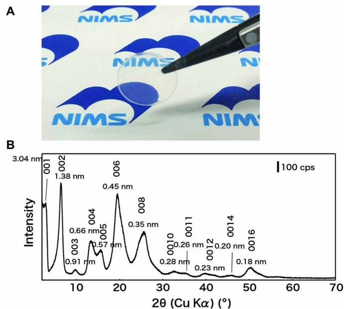
**Fig. 4. Zeolite film with a diameter of 18 mm obtained from the colloidal dispersion.** (A) photograph and (B) XRD data, which show only the basal reflections and no peaks associated with the in-plane periodicity, confirming that zeolite nanosheets are stacked with their faces parallel to the film surface. Photo credit: Yeji Song, NIMS.
