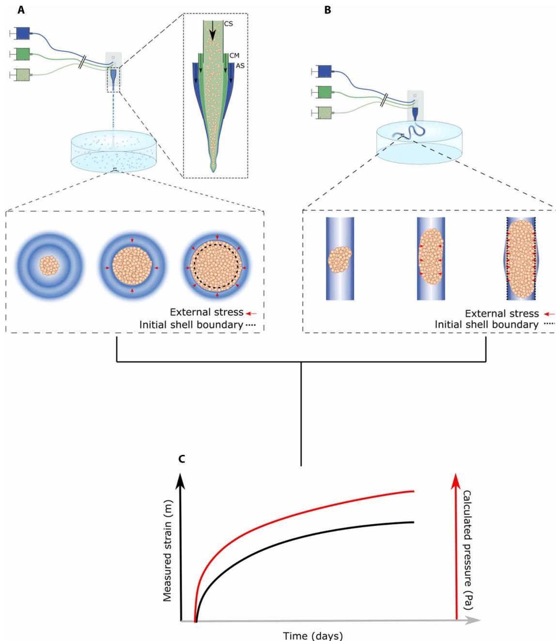
**Fig. 1. Experimental configuration.** (A) Coaxial coextrusion in air then alginate capsule stabilization within the calcium bath. (B) Coextrusion within the calcium bath allowing for formation of alginate tubes. (C) Experimental observation of the strain permits, knowing the mechanical properties of the alginate shell, to recover numerically the exerted pressure on tumor cell.
