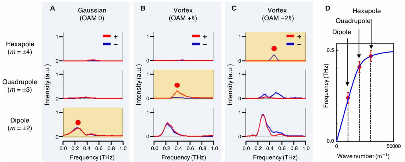
**Fig. 3. Mode decomposition of near-field distributions.** Frequency spectra of the dipole [ $E(\pm 2, f)$ ], quadrupole [ $E(\pm 3, f)$ ], and hexapole [ $E(\pm 4, f)$ ] modes excited in the sample illuminated by (A) Gaussian beam, (B) vortex beam ( $+\hbar$ ), and (C) vortex beam ( $-\hbar$ ). (D) Dispersion relation of the spoof LSP. The red dots represent the resonance frequencies determined in (A) to (C). The blue curve is a theoretical fitting.
