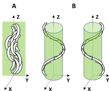
**Fig. 1. Schematic views of the structure of the modulated nematic phases formed by achiral bent-shaped molecules.** (A) In the splay-bend nematic phase, the director oscillates in a plane, chosen here to be the **YZ** plane of the laboratory frame **XYZ**. (B) In the twist-bend nematic phase, the director is arranged on a conical helix with doubly degenerate chirality. The helix axis, **h**, is parallel to the **Z** axis of the laboratory frame.
