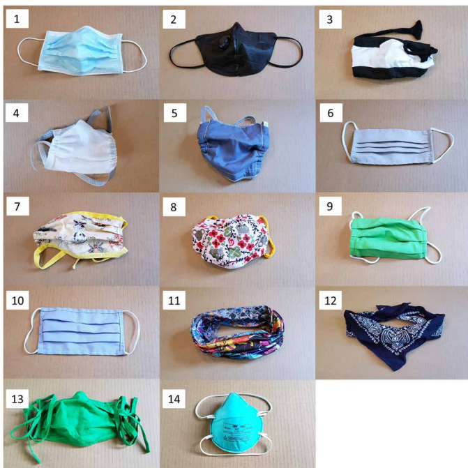
Fig. 2. Pictures of face masks under investigation. We tested 14 different face masks or mask alternatives and one mask material. Photo credit: Emma Fischer, Duke University. For photos showing the masks as actually worn, see fig. S8 (Supplementary Materials).
