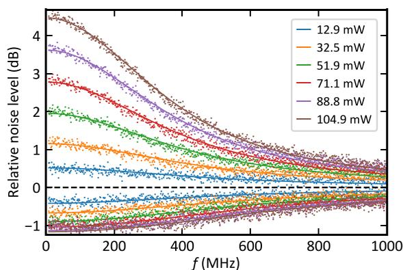
**Fig. 3. Squeezing and antisqueezing frequency spectrum from 20 MHz to 1 GHz at different pump power levels.** Powers listed are inferred values on-chip in the input waveguide. Dashed line is shot noise level; solid lines exhibit fits to the theoretical model (details in the Supplementary Materials), showing strong agreement with the measured data.
