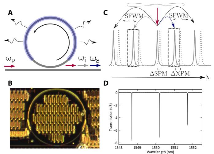
**Fig. 1. Overview of device.** (A) Schematic of microring device showing resonator, side channel, microheater (blue), and scattering modes. (B) Optical microscope image of device. (C) Illustration of intracavity SFWM process, showing frequency shifts  $\Delta\text{SPM}$  and  $\Delta\text{XPM}$  associated with self- and cross-phase modulation (SPM and XPM, respectively). (D) Representative transmission spectrum of microring device, showing three overcoupled resonances near 1550 nm.
