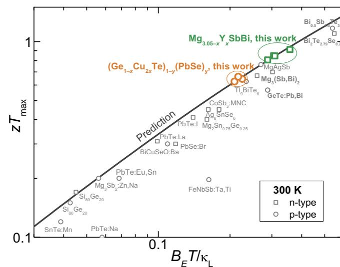
**Fig. 3. Thermoelectric quality factor  $B_E T / \kappa_L$  versus maximum  $zT$  ( $zT_{\max}$ ) at 300 K.**  $B_E T / \kappa_L$  is a good predictor for  $zT_{\max}$  of an optimally doped sample. The solid curve shows the prediction, and the symbols stand for measurements. Detailed references are given in fig. S5.
