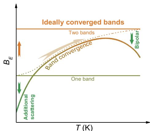
**Fig. 2. Schematic temperature-dependent  $B_E$ .** A model system involving a convergence of two identical bands, additional charge scattering, and a bipolar conduction.
