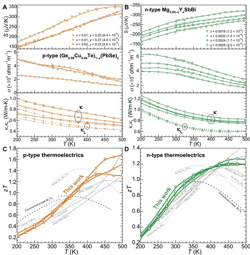
**Fig. 4. Thermoelectric properties.** Seebeck coefficient, electrical conductivity, thermal conductivity and its lattice component (A and B), and thermoelectric figure of merit  $zT$  (C and D) for p-type GeTe alloys and n-type  $\text{Mg}_3\text{SbBi}$  alloys, with a comparison to that of commercial  $\text{Bi}_2\text{Te}_3$  and other high-performance thermoelectrics (8, 9, 13, 14, 21–30) in the temperature range of 200 to 500 K.
