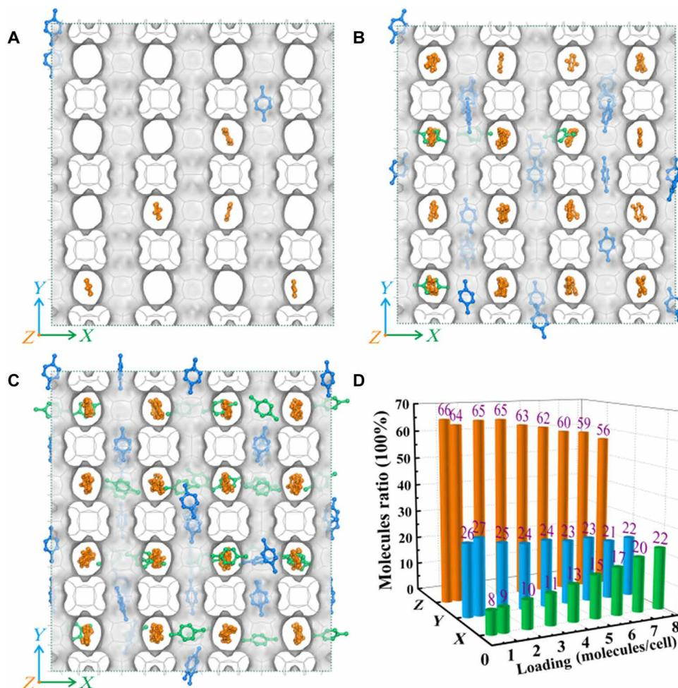
**Fig. 4. Channel occupancy in SCM-15 zeolite.** Adsorption sites of *p*-xylene inside the SCM-15 zeolite at (A) 0.5, (B) 4, and (C) 8 molecules per cell loading and at 298 K (obtained from MD trajectories; H atoms are omitted for clarity). (D) Molecular percentage of *p*-xylene molecules located in X, Y, and Z channels at different loading. Green, blue, and orange colors are used to indicate the locations of *p*-xylene in X, Y, and Z channels, respectively.
