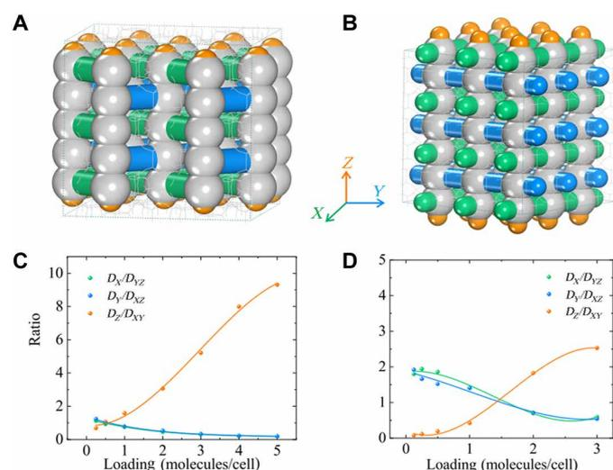
**Fig. 7. Channels and diffusion coefficients in POS and BEC zeolites.** 3D channels in (A) POS and (B) BEC zeolites. The silver balls represent intersections. The green, blue, and orange cylinders represent the channels along the X, Y, and Z directions, respectively. Variations in anisotropic diffusion coefficient ratio of *p*-xylene molecules as a function of loading in (C) POS and (D) BEC zeolites (298 K).
