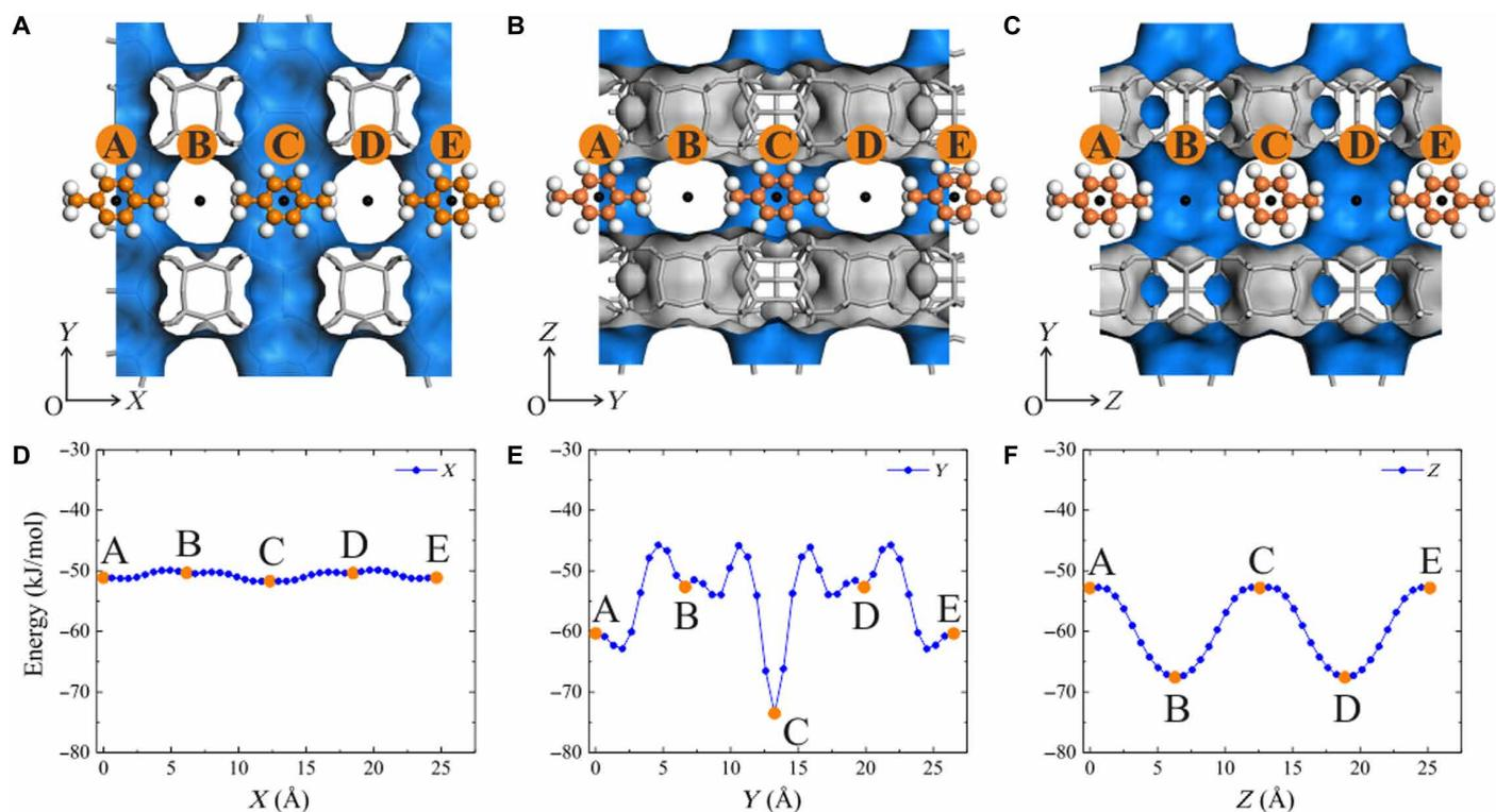
**Fig. 3. Diffusion pathways and interaction energy profiles.** Definition of *p*-xylene (center of mass) diffusion pathways (points A to E) along the (A) X, (B) Y, and (C) Z directions. The orange, white, and black balls represent C, H, and the center of mass of *p*-xylene, respectively. Interaction energy profiles of *p*-xylene along the (D) X, (E) Y, and (F) Z directions.
