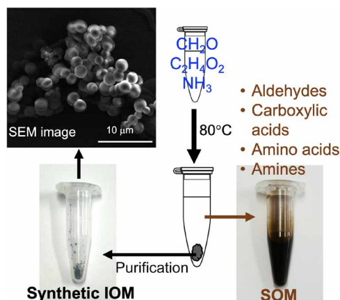
Fig. 1. AFR experiments and their products. Simple heating of formaldehyde, glycolaldehyde, and ammonia with calcium hydroxide formed amino acids, amines, carboxylic acids, and synthetic IOM. Photo credit for the scanning electron microscopy (SEM) image: Yoshinari Iwasa, Tohoku University. Photo credit for the synthetic IOM and SOM: Yoshihiro Furukawa, Tohoku University.
