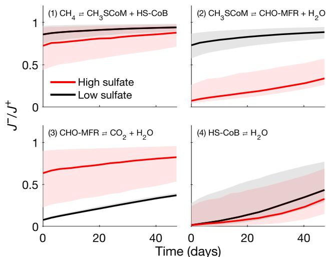
**Fig. 5. Individual reaction reversibility ( $J^-/J^+$ ) best fits to the experimental results.** The envelopes contain 68% of results based on  $10^5$  simulations with parameter values drawn from uniform prior distributions and weighted by the inverse of the sum of squared model-measurement mismatch ( $1/\text{SSE}$ ). The schematic chemical reactions in the panels show only the metabolites that participate in isotope exchange, and the full reactions are listed in Fig. 1.
