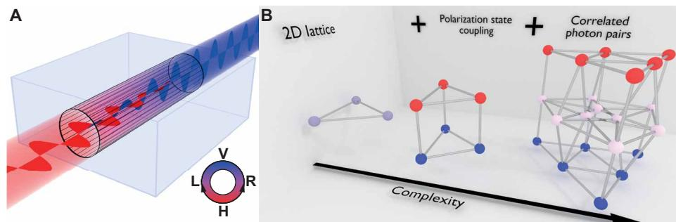
**Fig. 1. Using polarization as an additional synthetic dimension.** (A) A single waveguide with tailored birefringence coherently couples its horizontally (red) and vertically (blue) polarized modes of the electromagnetic field. (B) Planar graphs (left) acquire an additional dimension due to the coupling of two polarization states (middle). The Hilbert space of photon pairs on 3D graphs takes the form of a yet more complex graph (right).
