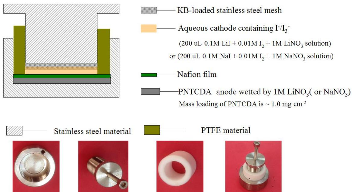
**Fig. S4. Schematically showing the assembly of full cell.** Detailed information and the photos of devices are given in above figure.
