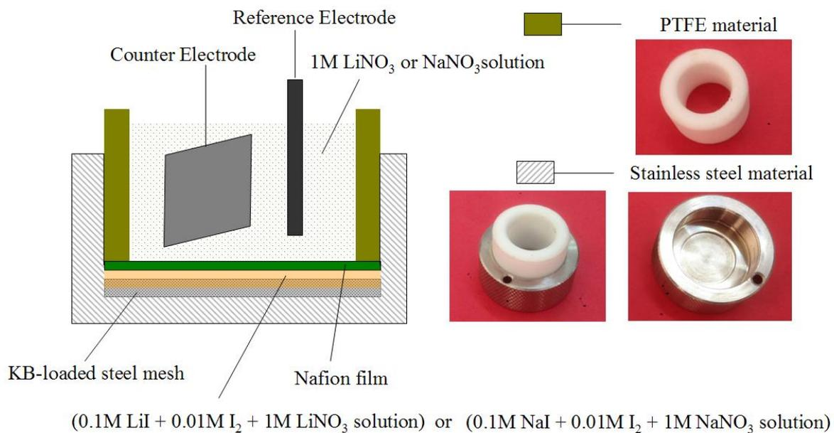
**Fig. S2. Schematic illustration of the cell for aqueous electrode investigation with a three-electrode system.**
