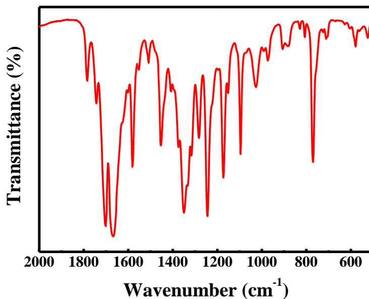
**Fig. S1. FT-IR spectrum of as-prepared PNTCDA.**
