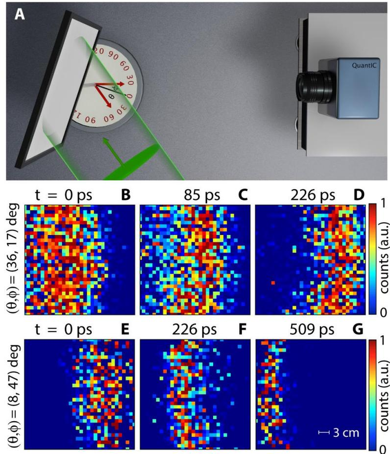
**fig. S4.** **A** shows a sketch of the experimental setup employed to perform the time-resolved imaging for the conditions reported above, with a SPAD camera detector. **B-D** show the images recorded for three different instant of time in case of subluminal propagation, whereas **E-G** show the same but for a superluminal scattering source.
