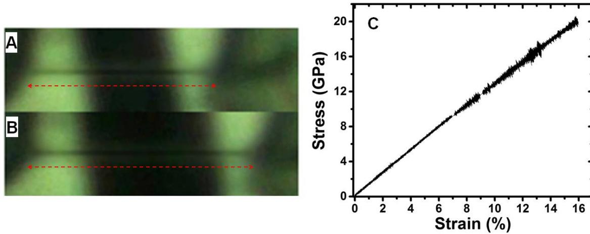
**fig. S1.** Monotonic tensile straining of a VLS-grown Si nanowire under optical microscope: (A), original status before test. (B), the status showing the maximum strain of ~16% (corresponding fracture stress ~20 GPa; the straining rate in this experiment was  $0.0017 \text{ s}^{-1}$ ). (C), the corresponding stress vs. strain curve (note that the contrast in the optical images was slightly enhanced).
