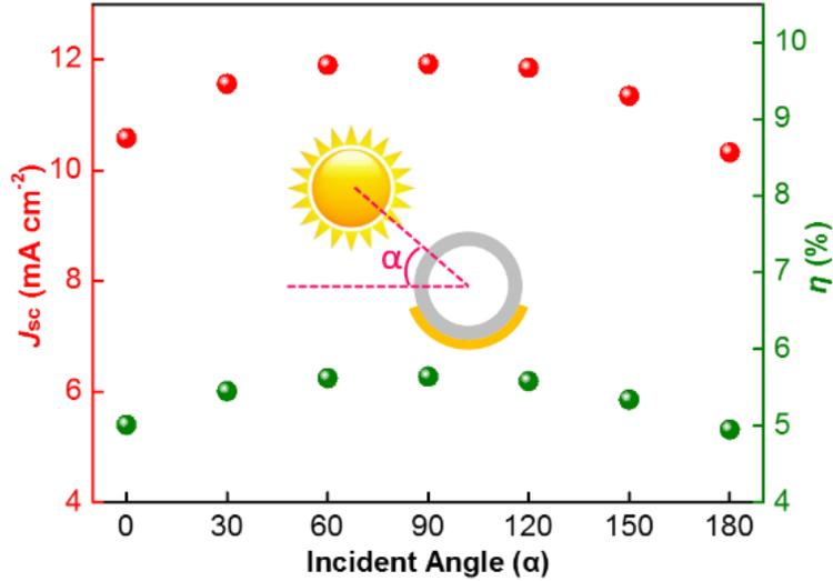
**fig. S4. Dependence of an F-DSSC under different incident light angles.** The schematic image of measuring the performance of single F-DSSC unit under different incident angles was shown as the inset.
