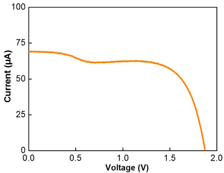
**fig. S8.  $I$ - $V$  curve of three F-DSSCs in series connection.**
