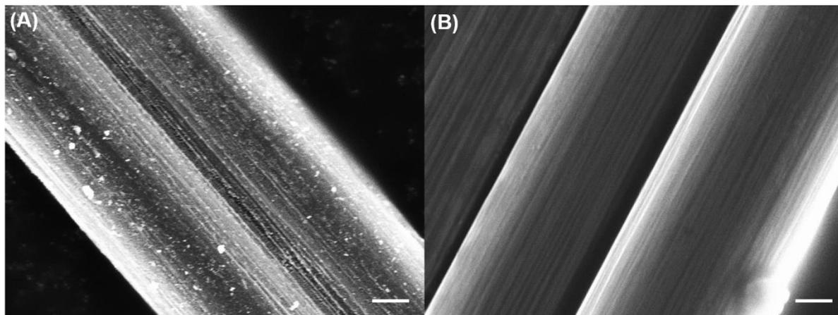
fig. S2. SEM images of pure carbon fiber and Pt-coated carbon fiber. Both of the scale bars are 2  $\mu\text{m}$ .
