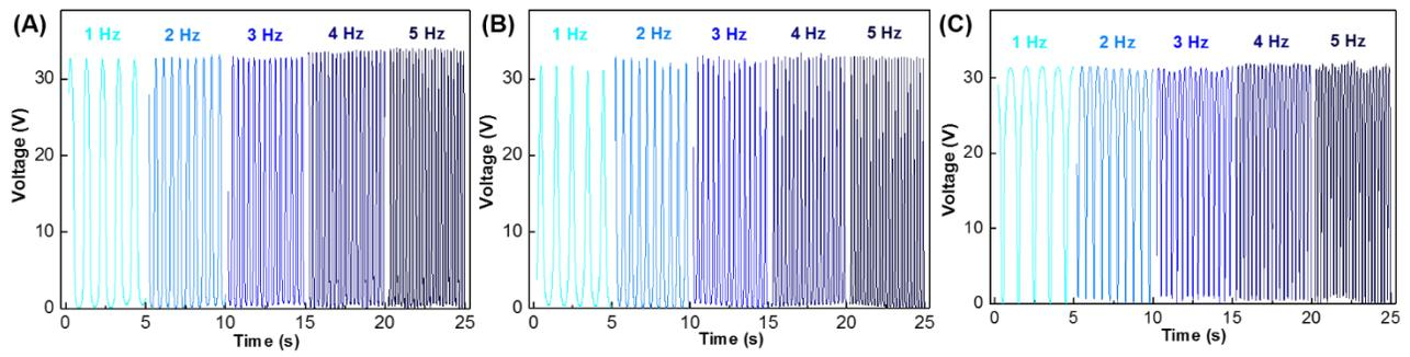
**fig. S7.  $V_{OC}$  outputs of F-TENG network textiles.** The open-circuit voltage outputs of F-TENG network textiles with knitting patterns of (A)  $1 \times 1$ , (B)  $3 \times 3$  and (C)  $5 \times 5$  nets at the frequencies ranging from 1 to 5 Hz.
