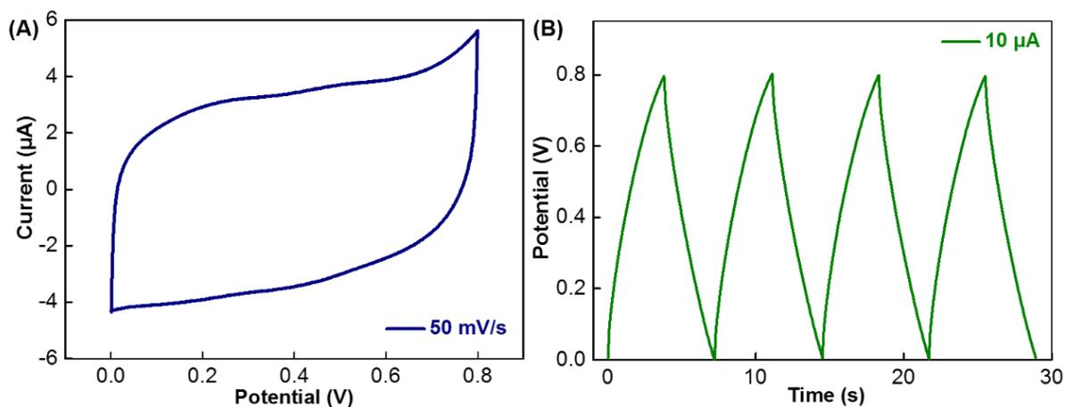
fig. S6. CV and GCD curves of an F-SC based on bare carbon fibers. (A) Cyclic voltammograms (CV) curve under the scanning rate of 50 mV/s and (B) galvanostatic charging/discharging (GCD) under current density of  $10 \mu\text{A}$  of a single fiber based supercapacitor based on bare carbon fibers.
