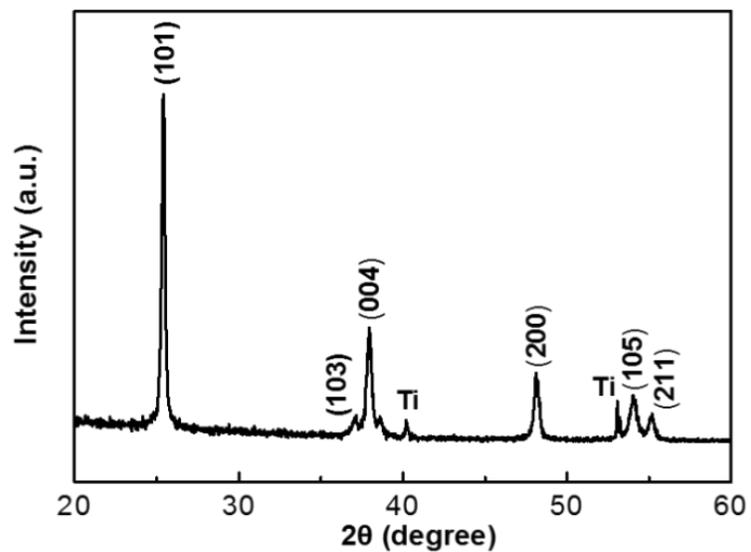
fig. S1. XRD pattern of the anodized  $\text{TiO}_2$  nanotube arrays on a Ti wire.
