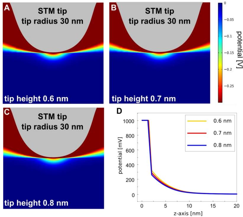
**fig. S1. Calculation (Poisson solver) of the tip-induced potential for varying tip heights above the GaAs surface. (A-C)** Spatial resolved potential (plotted color coded) for tip height of 0.6, 0.7 and 0.8 nm (doping density  $n_D=3e^{18}/\text{cm}^3$ , sample voltage 1.0 V, tip radius 30 nm). **(D)** Cross-sectional plot of the potential along the z-axis and in the middle of the STM tip.
