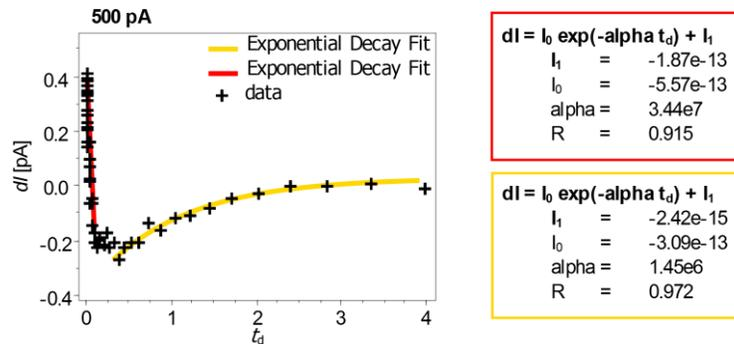
**fig. S4. Exemplary fitting results of the  $dI(t_d)$  spectra of Fig. 1E in the transition region.** In this case the fitting is restricted to early (red) and late (yellow) delay times. The parameter  $R$  stands for the nonlinear regression coefficient. The other parameters are self-descriptive.
