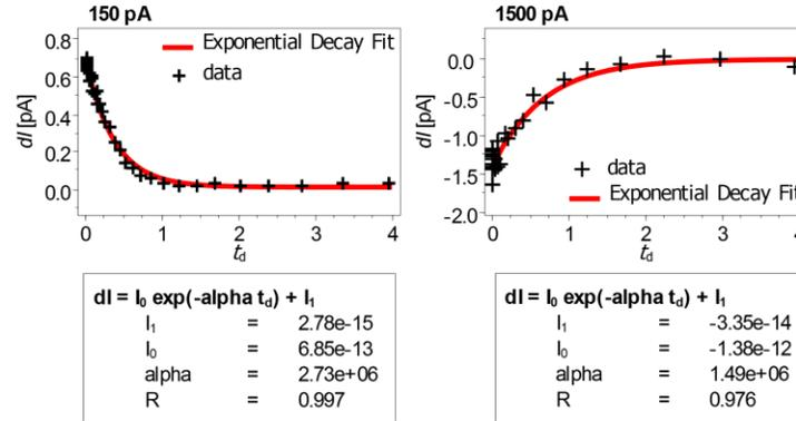
**fig. S3. Two exemplary fitting results of the  $dI(t_d)$  spectra of Fig. 1E.** The parameter  $R$  stands for the nonlinear regression coefficient. The other parameters are self-descriptive.
