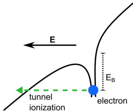
**fig. S8. Schematic for field-driven tunnel ionization.** The tunneling rate from the donor level into the conduction band is defined by the tip-induced electric field  $E$  at the dopant position and the binding energy  $E_B$ .
