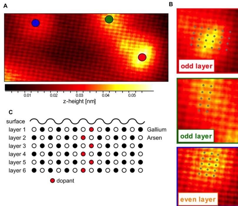
**fig. S6. Extracting the dopant depth from STM topographies.** (A) STM topography showing the signature of three buried dopants. Depending on the depth, the z-height modulation above the dopant decreases. (B) More detailed pictures of each single dopant labeled in red, green and blue in A. Grey points trace the atomic corrugation. (C) ABAB stacking at the GaAs(110) surface. Red dot: layer 1, Green dot: layer 3, Blue dot: layer 4.
