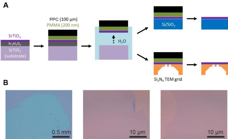
**fig. S2. Transfer of SrTiO<sub>3</sub> membranes.** (A) Schematic of SrTiO<sub>3</sub> layer release and transfer. During the sacrificial layer dissolution in water, the thick polymer layer functions as a mechanical support. (B) Optical images of transferred SrTiO<sub>3</sub> layers on oxidized Si (SiO<sub>2</sub> 300 nm) substrates, for 6 u.c. (left and center), and 4 u.c. (right). The measured AFM height profile well matches the thickness monitored by RHEED oscillations.
