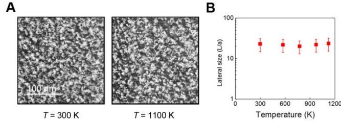
**fig. S5. In situ heating experiment in TEM.** (A) DF-TEM images of a 4 u.c. SrTiO<sub>3</sub> membrane at two different temperatures. (B) Crystalline domain size of a 4 u.c. SrTiO<sub>3</sub> membrane vs temperature.
