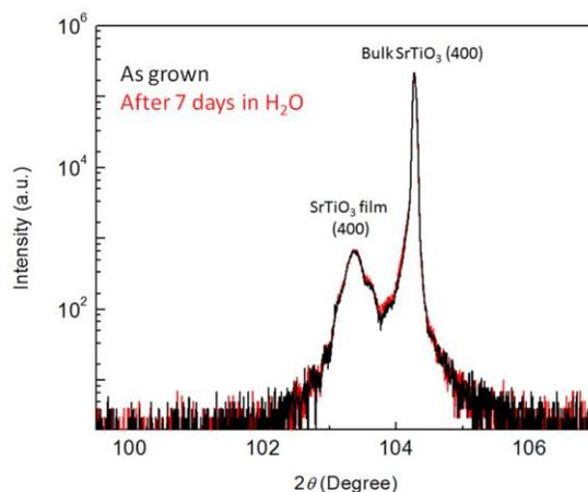
**fig. S3. Chemical stability of SrTiO<sub>3</sub> films.** XRD pattern around SrTiO<sub>3</sub> (400) of a 100 nm thick SrTiO<sub>3</sub> film grown on a bulk SrTiO<sub>3</sub> (100) substrate, before (black) and after (red) exposure to room temperature deionized water for a week. The SrTiO<sub>3</sub> film was grown slightly off-stoichiometry intentionally, in order to distinguish the film peak from the bulk substrate peak. The two film XRD peaks before and after exactly overlap each other.
