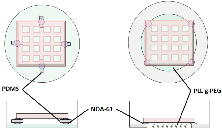
**fig. S5. Illustration of the scaffold fabrication method.** Top: schematic of the master fabrication, with PEG-DA photopolymer (red) between an acrylated glass slide (light blue) and a fluorosilanized coverslip (blue) fixed together by tape (green). Middle: The final polymerized master after removing the coverslips. Bottom left: functionalized PDMS scaffold attached to a standard 6-well plate. Bottom right: functionalized PDMS scaffold attached to a passivated glass bottom dish.
