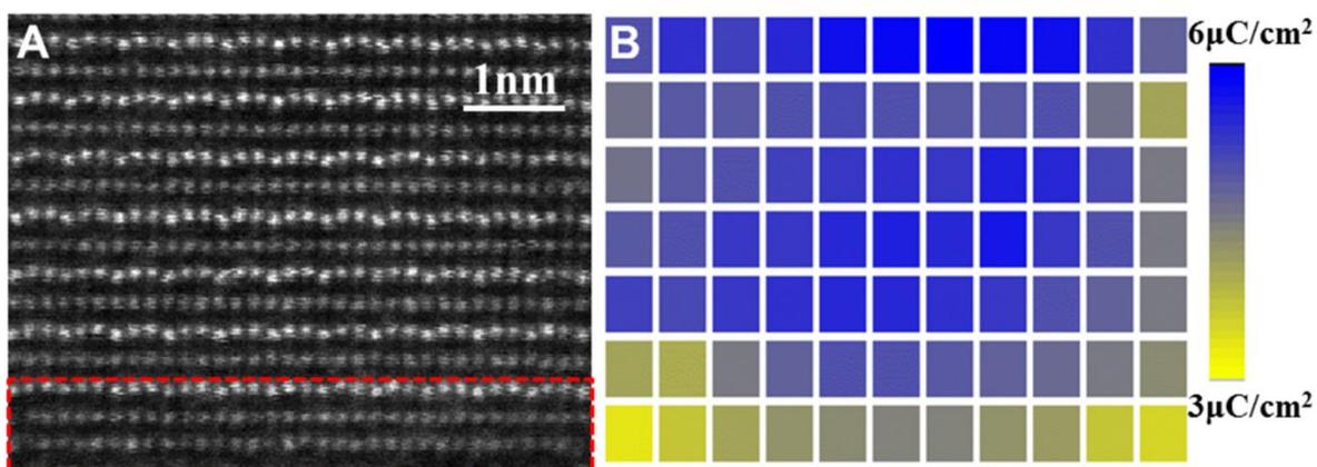
**fig. S2. Quantitative evaluation of polarization in the film.** (A) STEM image used for polarization mapping. Modified from Fig. 1D in the main text. (B) Calculated ferroelectric values from STEM image. Each box represents up-up-down polarization unit and the color represents the polarization value.
