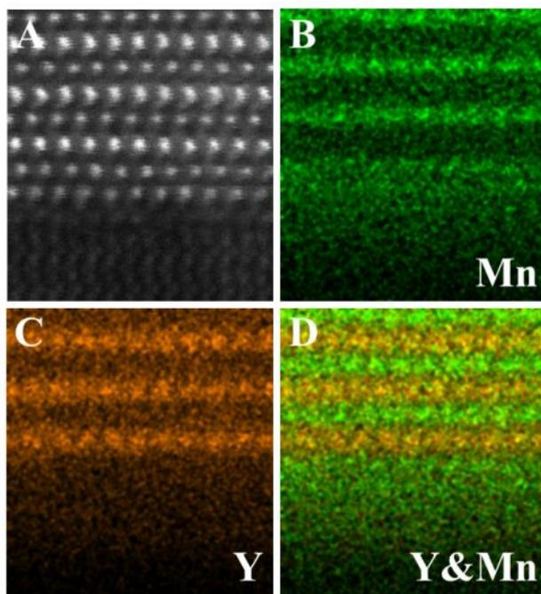
**fig. S3. EDS mapping results for the interface.** (A) HAADF image for the interested interfacial area. (B) Mn element mapping. (C) Y element mapping. (D) Combination of Y and Mn signals.
