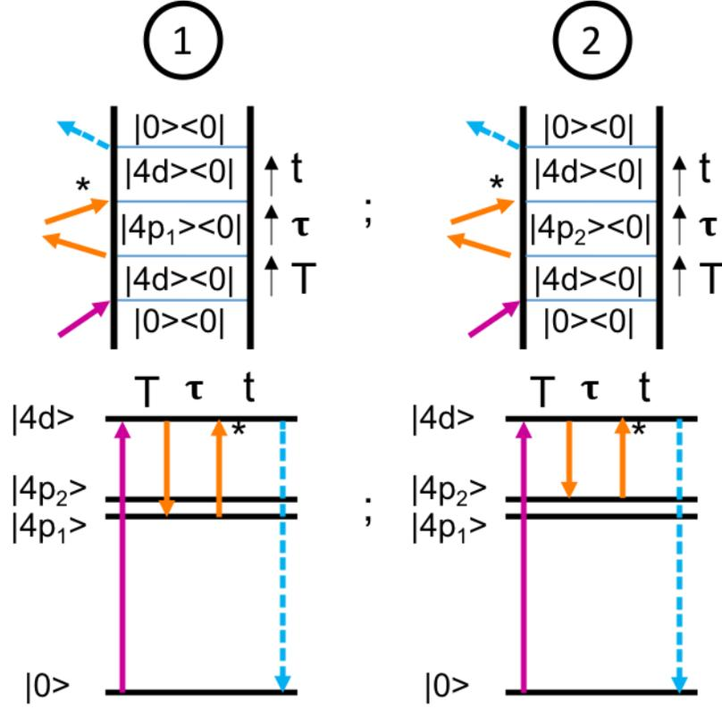
**Fig. S1. Double-sided Feynman and Jablonski diagrams of two interfering pathways.** The shaped NIR pulses considered in the derivation are indicated by the asterisk.
