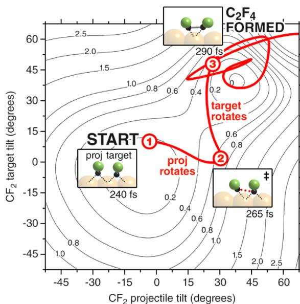
**Fig. S6. Trajectory for direct association reaction superimposed on a restricted cut through the ground potential energy surface.** The cut was obtained by calculating the potential energy of independently rotated CF<sub>2</sub> projectile and CF<sub>2</sub> target, while the distance between the two CF<sub>2</sub>
