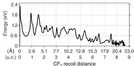
**Fig. S2. Distance dependence of the energy in the recoiling  $\text{CF}_2$ .** The energy shown is the sum of the translational and rotational energies of  $\text{CF}_2$  in the I2S trajectory shown in fig. S1 and movie S1.
