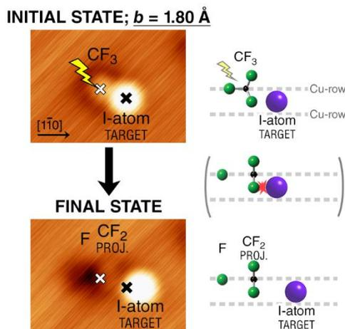
**Fig. S4.  $\text{CF}_2 + \text{I}$  collision at  $1.80 \text{ \AA}$  impact parameter, giving only momentum transfer from the projectile to the target.** STM images and schematics showing the initial and final state of
