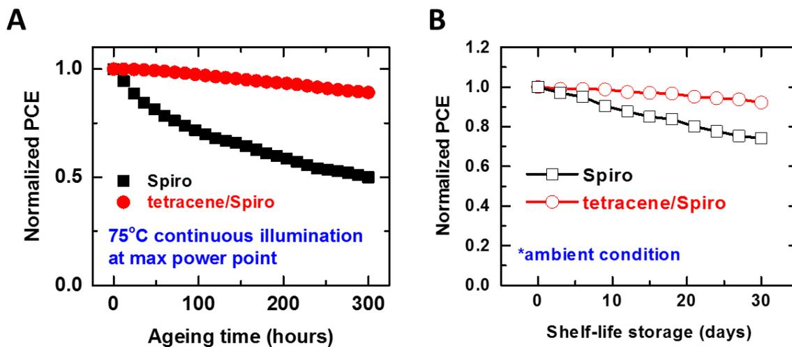
**Fig. S6. Device stability.** (A) Stability curve of the solar cells at maximum power point under continuous AM 1.5 G illumination, N<sub>2</sub> atmosphere and stabilised temperature of 75 °C. (B) Shelf-life of devices stored in ambient condition over a month and tested regularly under full AM1.5 simulated sunlight.
