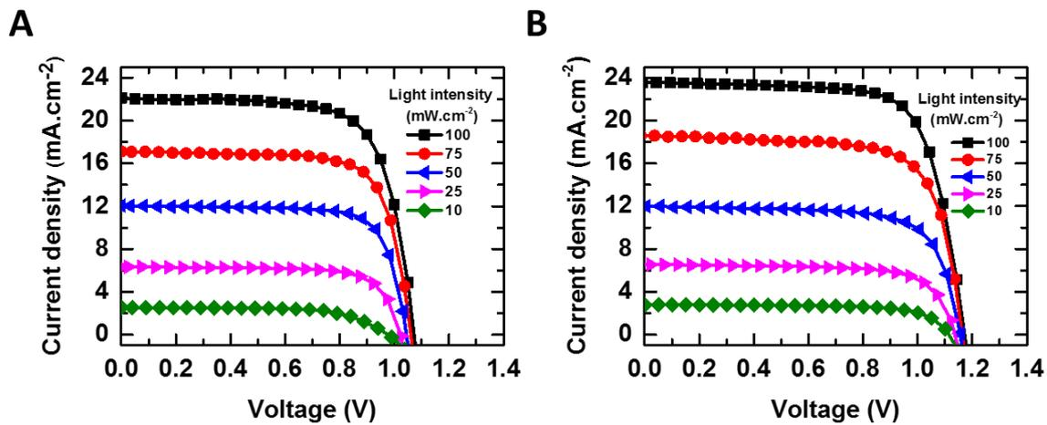
**Fig. S7. The current-voltage characteristic as a function of light intensity for PSCs with different HTL configurations. J-V characteristics of solar cells with (A) Spiro and (B) Tc-Spiro HTLs under different light intensities.**
