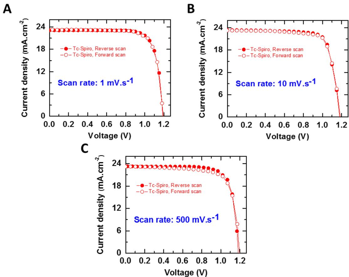
**Fig. S5. Hysteresis behavior of graded doped HTL-based PSCs at different scan rates.**
