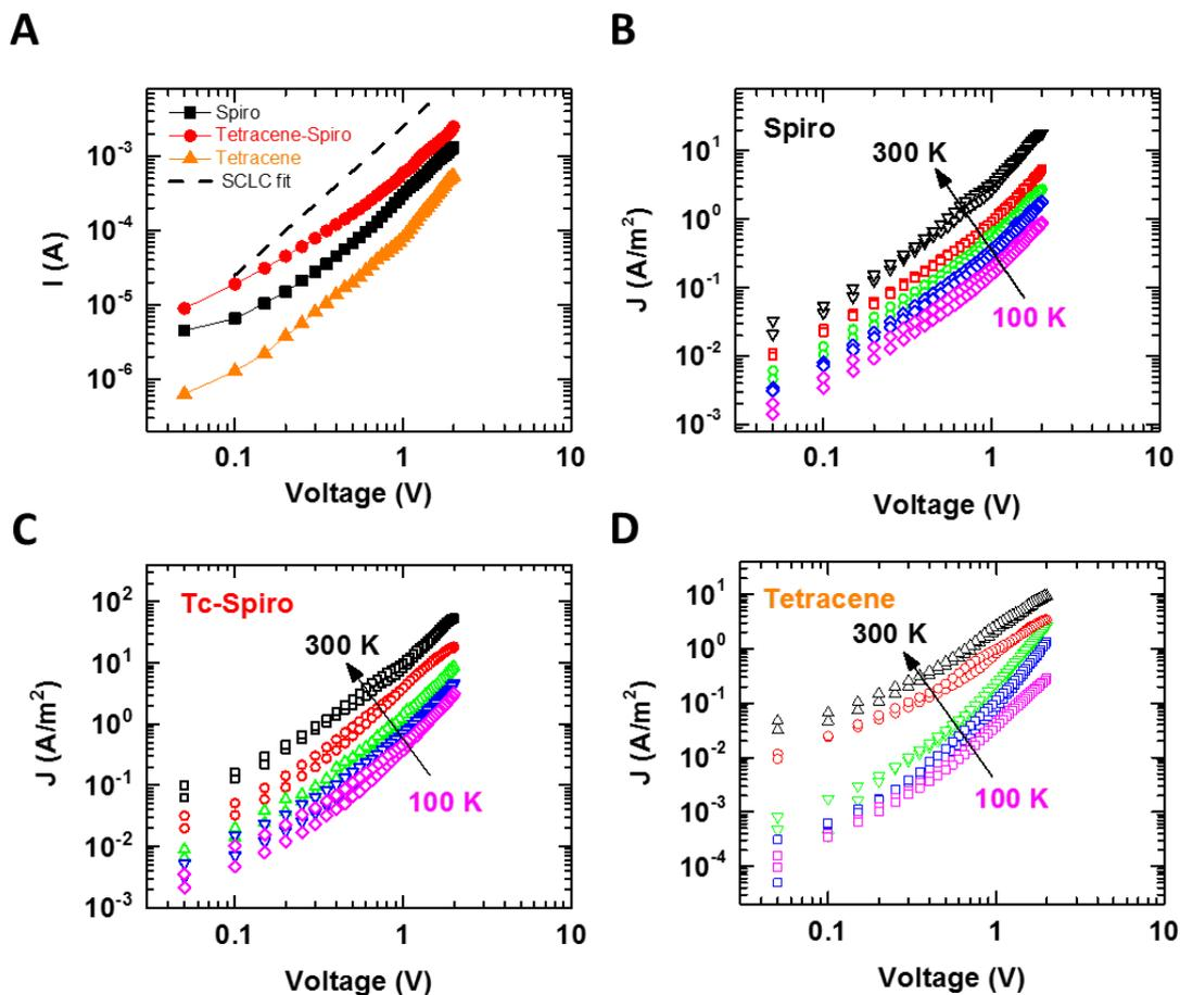
**Fig. S8. Temperature-dependent SCLC charge transport characterization of hole-only PSCs.** (A) I-V characteristics of hole-only perovskite devices with different HTL configurations measured at room temperature. I-V characteristics of (B) Spiro, (C) Tc-Spiro and (D) tetracene hole only devices (FTO/perovskite/HTL/Au) at different temperatures, utilized for estimating the space charge limited activation energy for hole transport. The temperature gradient between each curve is 50 K.
