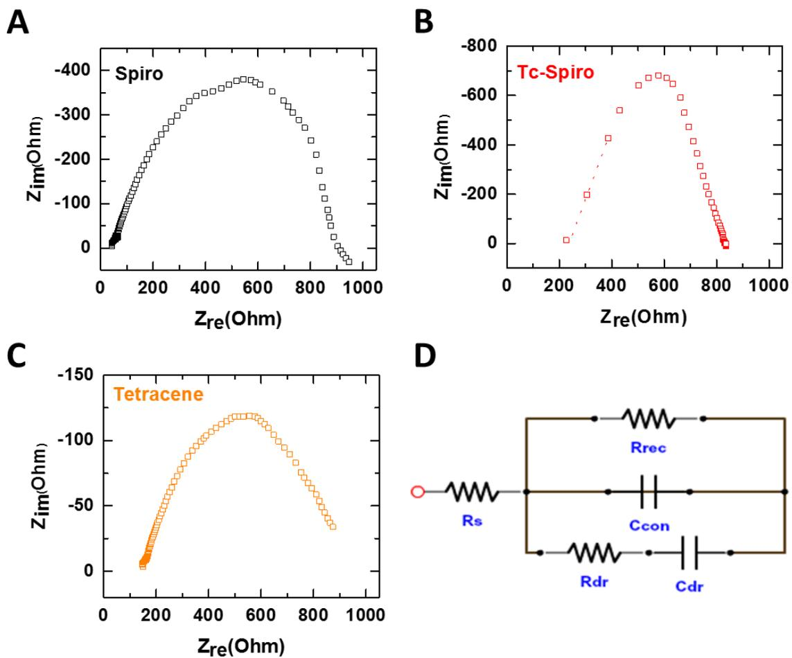
**Fig. S9. EIS of PSCs with different HTL configurations.** Typical EIS spectra measured on the perovskite solar cells with (A) Spiro, (B) Tc-Spiro and (C) tetracene as HTL. (D) Equivalent circuit for electrochemical impedance spectroscopy (EIS) measurement.
