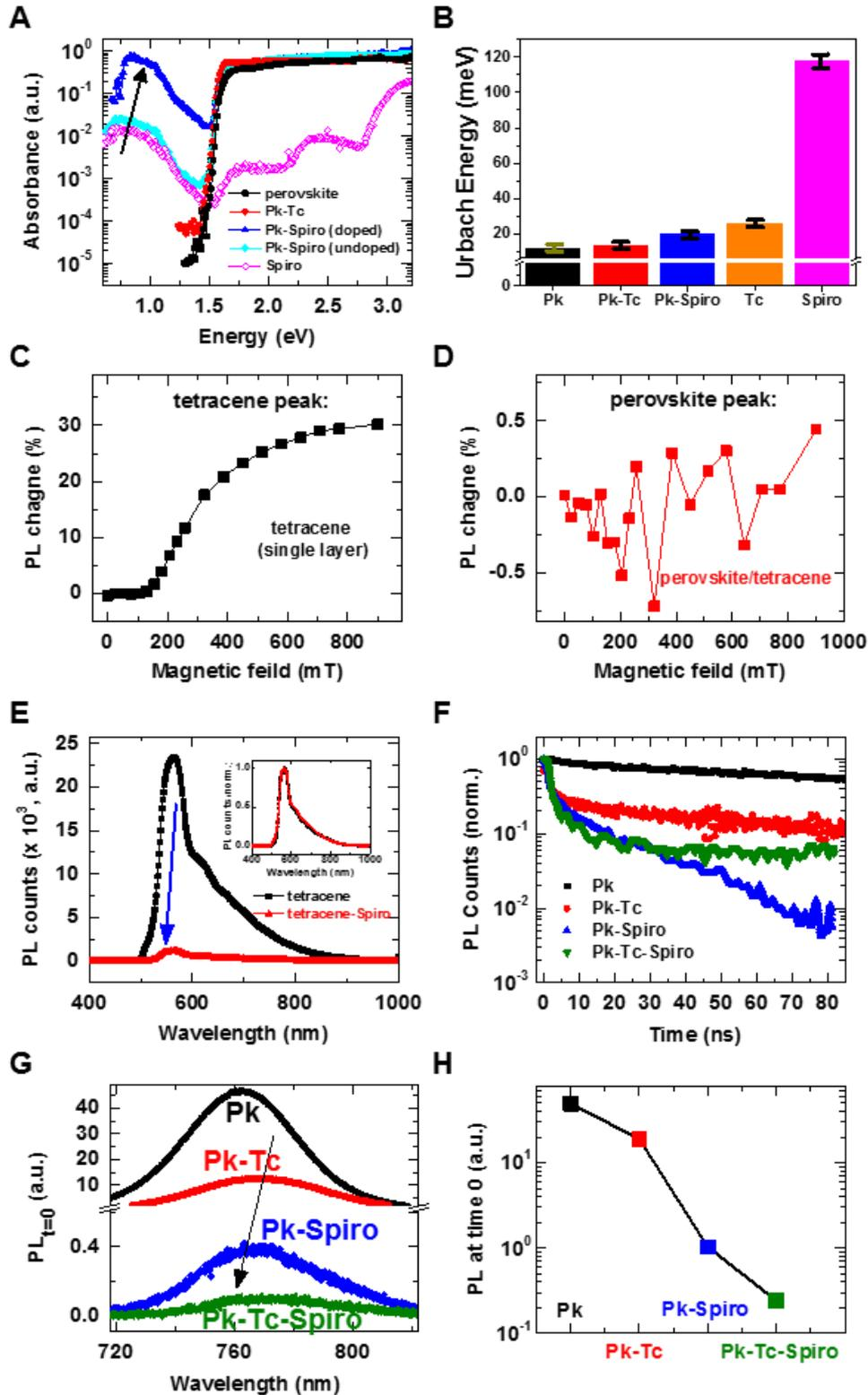
**Fig. S2.** Optical and magnetic field characterization of the perovskite thin films interfaced with a different configuration of HTLs. (A) PDS absorption spectra of perovskite, perovskite/doped-Spiro, perovskite/un-doped Spiro and Spiro thin films. (B) The
