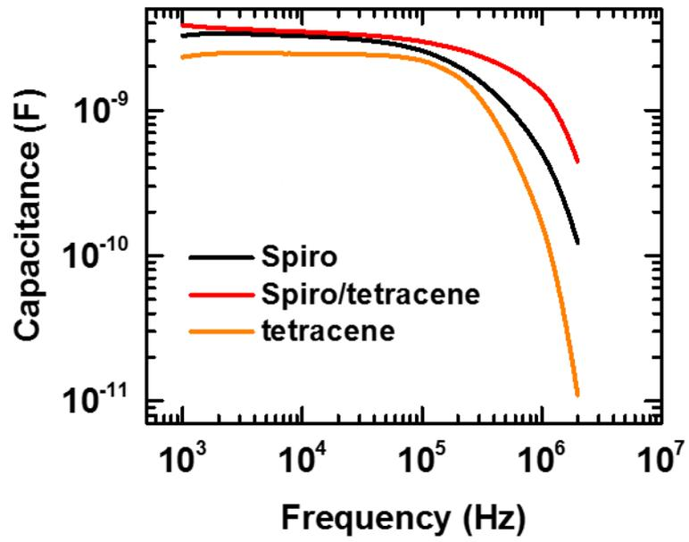
**Fig. S10.** Typical capacitive response of the perovskite layers interfaced with different HTLs.
