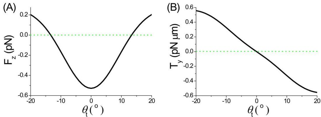
**Fig. S4. Robustness of OPF versus orientation.** Optical pulling force  $F_z$  (A) and restoring torque  $T_y$  (B) versus the tilted angle  $\theta_t$  around y-axis. An azimuthally polarized Bessel beam with a central ring power of 1 mW and a half cone angle  $30^\circ$  illuminates the cylinder of diameter 600nm and length 1500nm.
