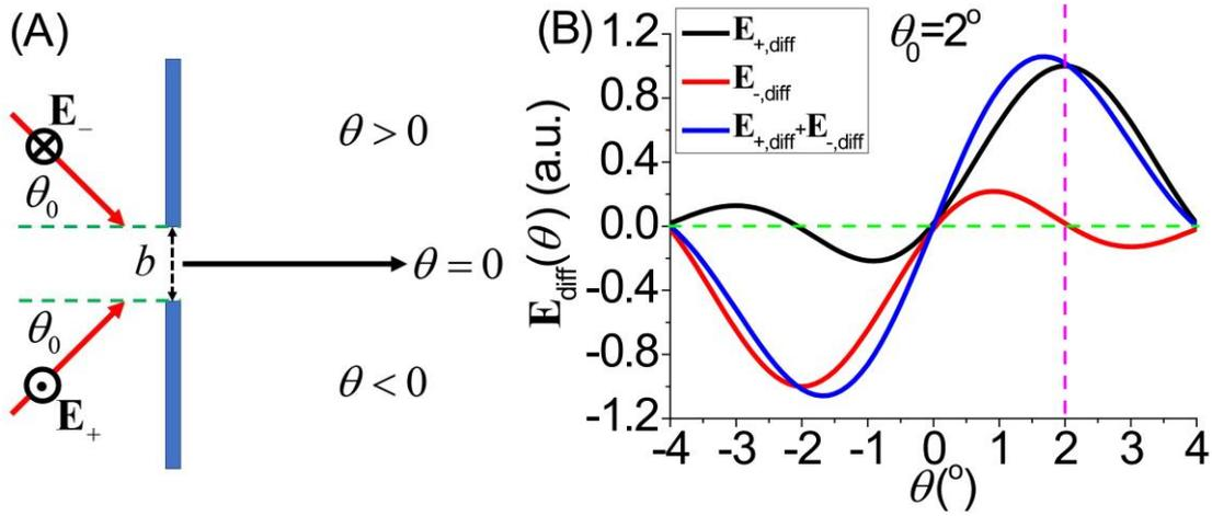
**Fig. S2. Collimation of two nearly forward propagating plane waves through single-slit diffraction.** (A) Illustration of a single slit diffraction when two out-of-phase incident plane waves illuminate on it at angle  $\theta_0$ . The slit has a width of  $b(\theta_0)$ . (B) Diffracted fields versus  $\theta$  for  $\mathbf{E}_+$ ,  $\mathbf{E}_-$ , and  $\mathbf{E}_+ + \mathbf{E}_-$ .
