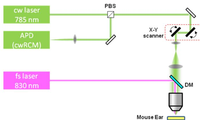
**Fig. S3. Schematic of the point treatment system.** The fs laser and the cw laser are combined with a dichroic mirror (DM) located before the objective lens. APD, avalanche photodiode; PBS, polarized beam splitter.
