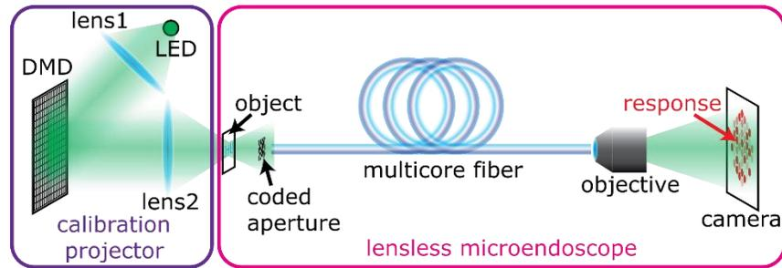
**Fig. S1. Detailed schematic of our approach consisting of calibration optics and the imager.**
