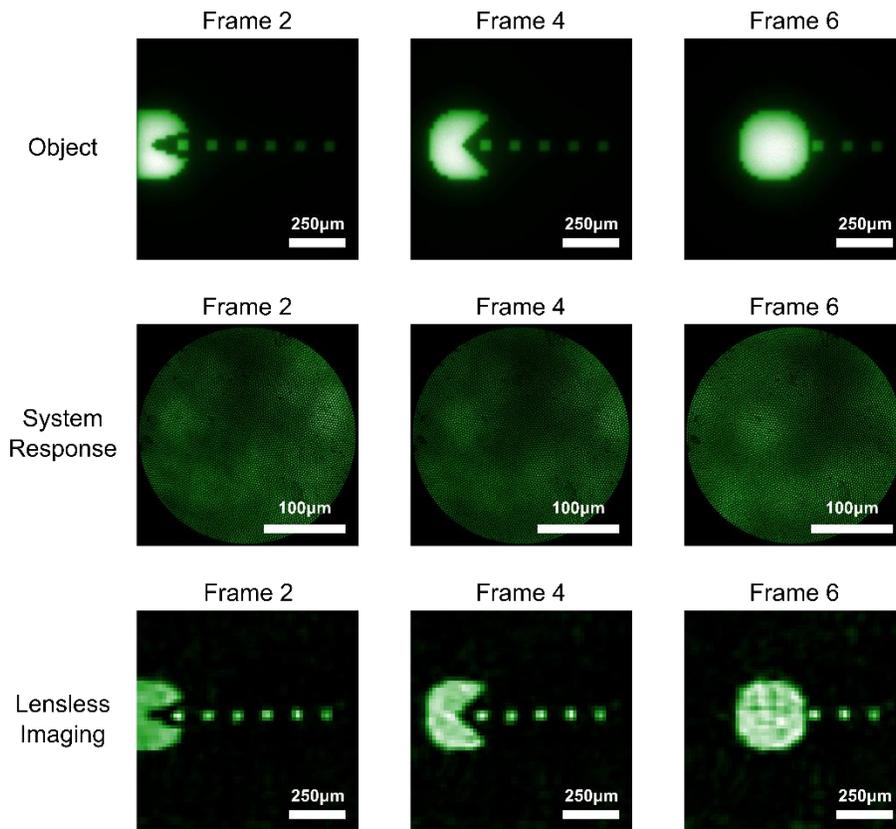
**Fig. S5. Demonstration of time-varying scene reconstruction.** A moving object is generated using the DMD from fig. S1 and imaged using a lens and a camera. The lensless microendoscope system responses for different frames are acquired at 50 frames per second using the CCD camera and used to reconstruct the scene. A movie of entire 14 frames is included.
