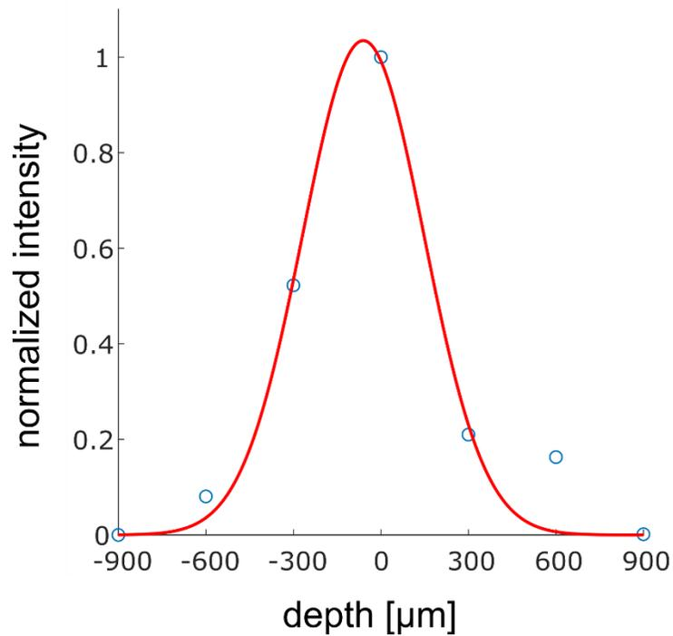
**Fig. S2. Determining the axial resolution of the lensless microendoscope.** An experimental point source is reconstructed at different depths and the corresponding intensity fall-off is recorded as a function of depth. A fitted Gaussian curve shows that the axial resolution is approximately 300  $\mu\text{m}$  according to the Rayleigh criterion.
