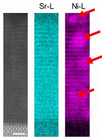
**Figure S2.** HAADF STEM image (left, scale bar is 2 nm) and corresponding individual EELS maps (right) for the Sr  $L_{2,3}$ , and Ni  $L_{2,3}$  ionization edges at lower magnification. The red arrows show some NiO clusters existed in the SNO films.
