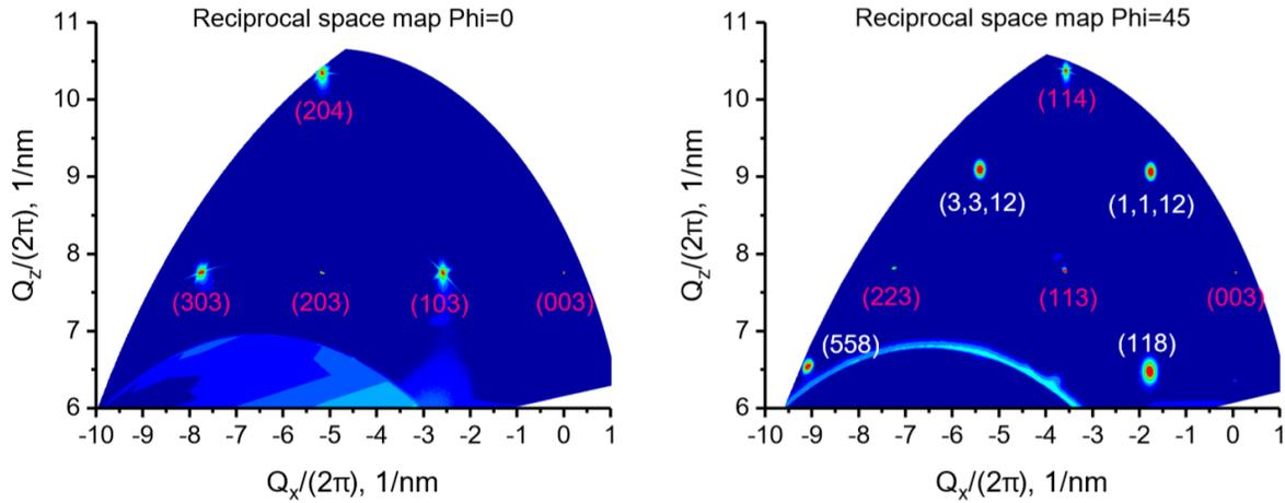
**Figure S1.** Wide-range RSM for 25 nm SNO/LSAT(001) measured along  $\phi = 0^\circ$  and  $\phi = 45^\circ$ , where x corresponds to the [100] direction (left) and [110] direction (right) of the LSAT substrate, z corresponds to the [001] direction. The film and substrate peak indices are written in white and purple, respectively.
