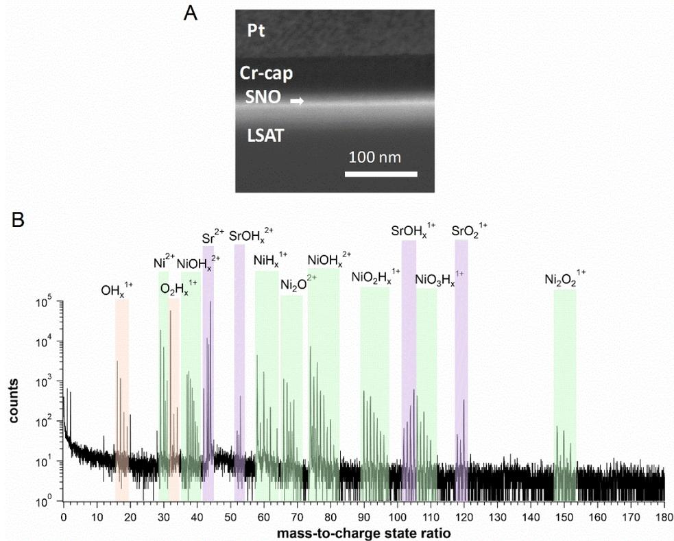
**Figure S4.** Cross-sectional view of SNO/LSAT sample in SEM and Mass spectrum. **(A)** Cross-sectional view of SNO/LSAT sample in Scanning electron microscope (SEM). **(B)** Mass spectrum of SNO films from atom probe tomography (APT) highlighting the assignment of ionic species.
