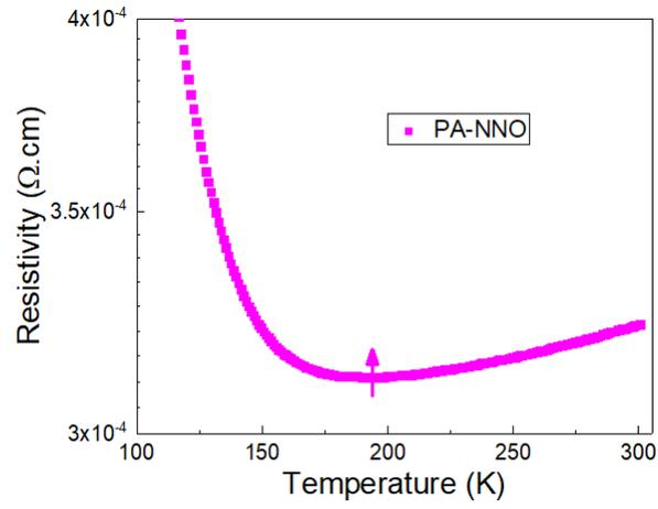
**Figure S5.** Temperature dependent resistivity of PA-NNO. The purple arrow denotes the metal-insulator transition point ( $T_{MI}$ ).
